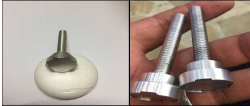
a) Modified Stub b) standard stub Plate 1; types of stubs.
